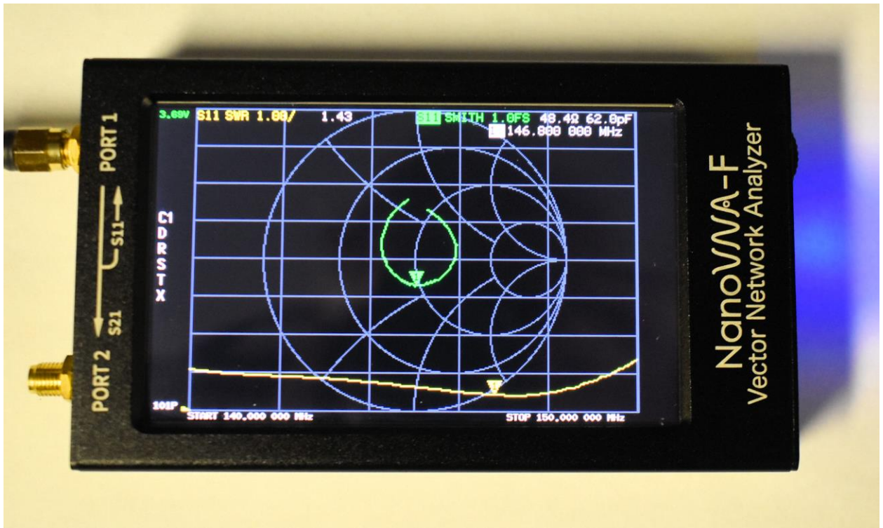
Tape Measure Antenna Smith Chart showing Impedance and Inductance
