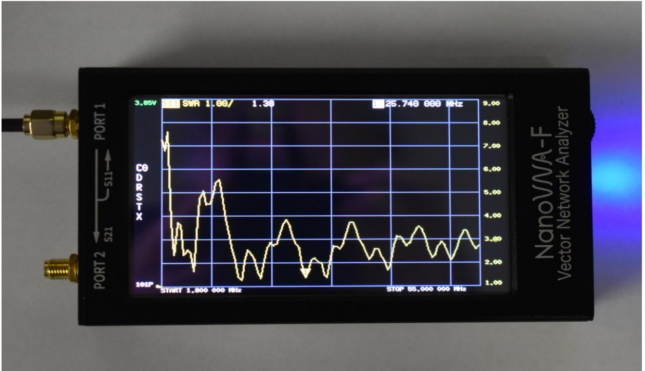
SWR plot for 80 meter OCF Dipole – marker at 15 meter band
